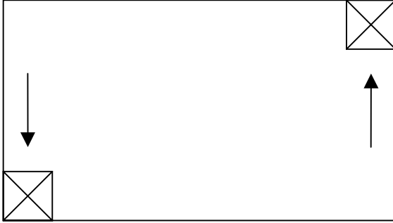
Fig. 1. Workplace with access to two stairways.
